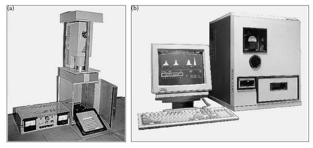
Figure 2. View of the X-ray apparatus (a), and the SKCS (b)
