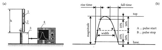
Figure 6. Scheme of the used apparatus (a): 1 – barley kernel, 2 – glass tube, 3 – force transducer, 4 – digital oscilloscope (DSO): and graphic presentation of the pulse parameters and their geometric sense (b)
