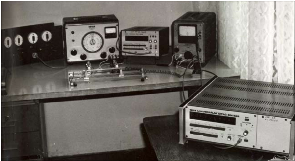
Figure 2. The comprehensive view of the measurement instrument at the transverse oscillations of a stem sample
