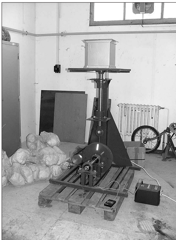
Figure 1. Testing stand of RIAE Prague for samples mechanical loading examination (mechanical loading motion simulator)
