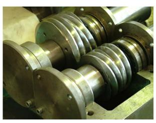
Figure 8. Helical gearing after test by loading 7<sup>th</sup> stage
