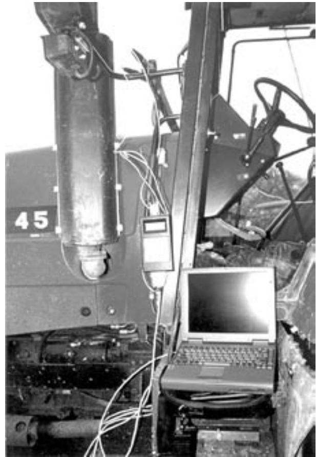
Fig. 2. Transmission of measuring data from recording units HMG 2020 to PC MicroBook 825D
