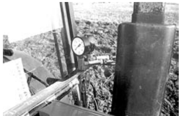
Fig. 3. Placement of the pressure tested transducers in the cabin of the tested tractor
