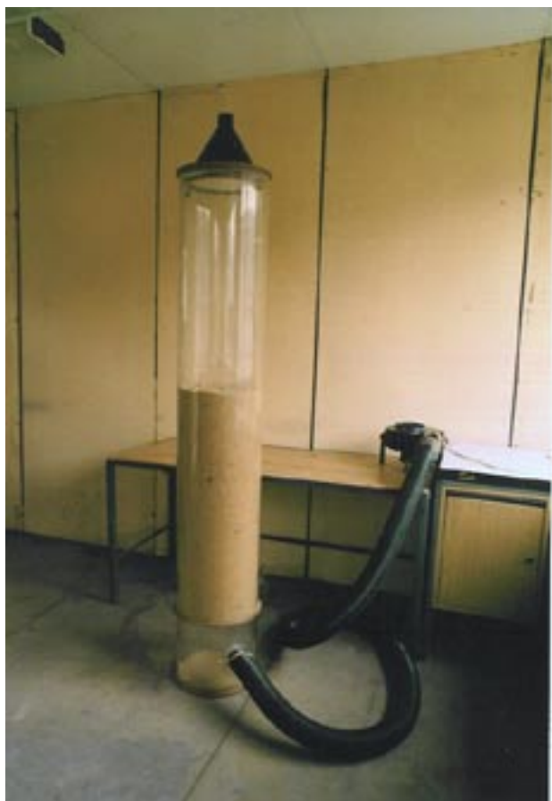
Fig. 1. The device for measurement of pressure drops in a dried material layer
