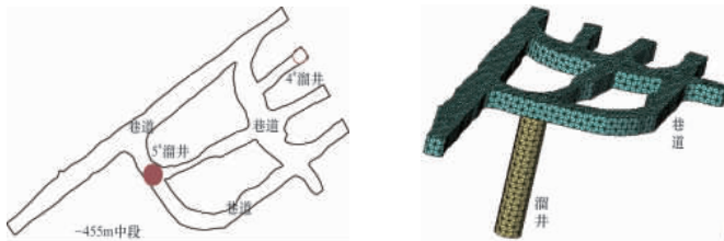
(a) -455m 中段溜井和巷道位置 (a) -455m middle part ubiety of roadway and ore pass (b) 有限元分析模型 (b) Finite element analysis model
