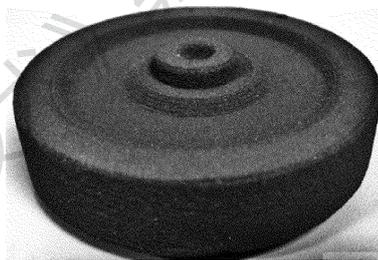
Fig. 1 Turbine part after SLS
