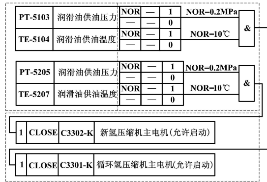
图 2 循环氢/新氢压缩机开机逻辑图 Fig. 2 Startup logic of the recycle/fresh hydrogen compressor
