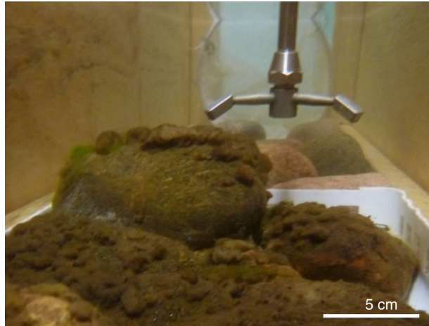
Fig. 4 Photograph facing downstream in the flow chamber with rocks covered in thick healthy mats of D. geminata taken from the Deer Creek site during the September 2011 shear removal tests (DC1). Note the ADV and the plankton net in the background used to collect any material removed due to the increasing applied bed shear stress.
