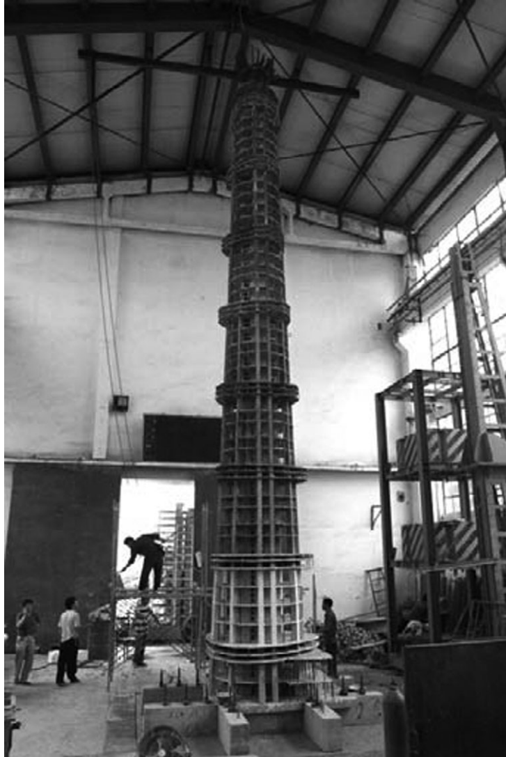
Figure 1. Shaking table test model of Shanghai center tower.
