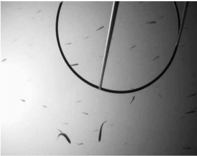
Fig. 4. Still from the video recording during temperature microstructure profiling for the profile shown in Fig. 3c. The circular construction in the upper part of the picture is part of the sensor guard at the microstructure profiler.
