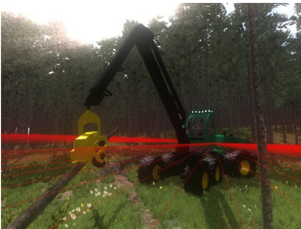
Figure 10 A Virtual Testbed with a harvester using door-mounted laser scanners to generate a local tree map
