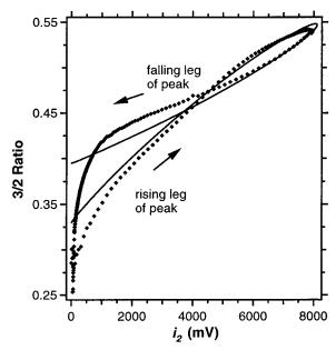
**Figure 5.** Instantaneous  $i_3/i_2$  ratios collected across a single peak. Each point represents an individual pair of background-corrected  $i_2$  and  $i_3$  measurements. Solid line is the calculated ratio for a Gaussian peak with width (4 $\sigma$ ) of 10 s, amplifier time constant of 1.3 s, K = 24 ppm mV<sup>-1</sup>, and true  $i_3/i_2$  ratio of 0.33.
