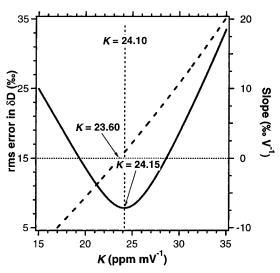
**Figure 3.** Comparison of H<sub>3</sub> factors determined by three methods for a typical *n*-alkane analysis. Vertical dotted line gives the value of *K* obtained by the bellows method. *K* is determined by the peak-rms method as the minimum in the  $\delta$ D error vs *K* curve (solid line). *K* is determined by the peak-slope method where the slope of the regression of  $\delta$ D error on peak height is zero (dashed line).
