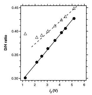
**Figure 2.** Typical "H<sub>3</sub> plot" used to calculate the value of *K*. Uncorrected data (triangles) are nonlinear because of mixing between the sample gas and background signals. After correcting for background ion currents, a linear relationship is obtained (circles). Note that the use of uncorrected data to determine the value of *K* will result in erroneously low values (dashed line with lower slope).
