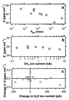
**Figure 6.** Changes in the value of *K* associated with He (a), CH<sub>4</sub> (b), and H<sub>2</sub>O (c) background signals. In panel c, relative changes in the value of *K* are plotted against changes in H<sub>2</sub>O<sup>+</sup> ion current over the same interval in order to remove the effects of instrumental drift.
