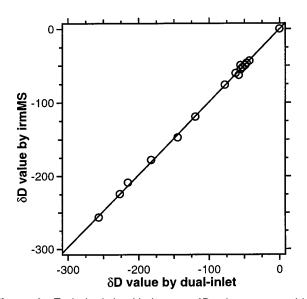
**Figure 6.** Typical relationship between  $\delta D$  values measured by conventional dual-inlet versus isotope ratio monitoring techniques. Least-squares regression of these data gives y = 0.987x - 0.6, with  $r^2 = 0.9988$ . The solid line is y = x and is indistinguishable from the regression line at this scale.
