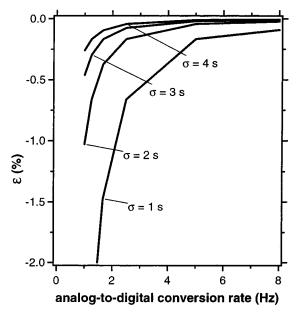
**Figure 5.** Estimated values of  $\epsilon$  as a function of peak width and analog-to-digital conversion frequency. All data are for Gaussian-shaped peaks ( $\sigma$  = standard deviation) with no background H<sub>2</sub> signals.
