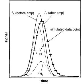
**Figure 1.** Typical output from the simulation of a Gaussian peak.  $H_{3}^{+}$  and HD peaks are offset due to isotope chromatography. The sample peak is broadened by the existence of a 1.3-s time constant in the signal amplification circuit.
