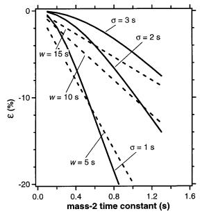
**Figure 4.** Estimated values of  $\epsilon$  as a function of peak width and mass-2 time constant. Data are for Gaussian (solid lines;  $\sigma$  = standard deviation) and rectangular (dashed lines; w = width) peaks with no background H<sub>2</sub> signals.
