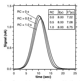
**Figure 3.** Decrease in the area under the square of signal intensity when peak shape is broadened by electronic time constants. All three curves represent the same 10-s-wide Gaussian curve filtered by three different time constants. This decrease in the ratio of integrated areas leads to an underestimate of  $H_3^+$  contributions.
