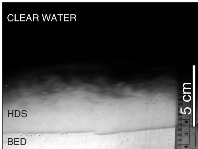
FIG. 3.—Photograph of the high-density suspension from experiment S9. The sediment was white. The lighting was from below and at an angle to maximize the visibility of the HDS. The clear water region above the HDS was dilute in comparison to the HDS, but still had sediment concentrations of \sim 2\text{--}3 \text{ g/l} (Table 1). Note the strong turbulent deformation in the HDS and the patchiness of the suspended sediment. The actual patchiness was greater than what appears in the photograph because of smearing during the exposure time.
