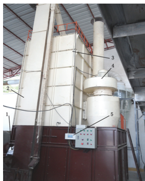
注: 1. 水分检测仪; 2. 提升机; 3. 干燥机; 4. 引风机; 5. 控制器 Note: 1. Online detector of grain moisture; 2. Conveyor; 3. Dryer; 4. Induced draft fan; 5 Controller
