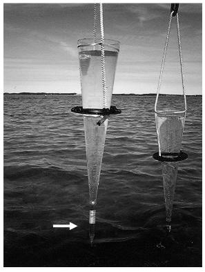
Fig. 1. Apparatus for collecting marine aggregates in shallow coastal habitats with soft substrates. A 15-mL Falcon tube (arrow) was secured to the bottom of a 1-liter settling cone, which was hung from a sheppard's hook using a ring-rope harness.
