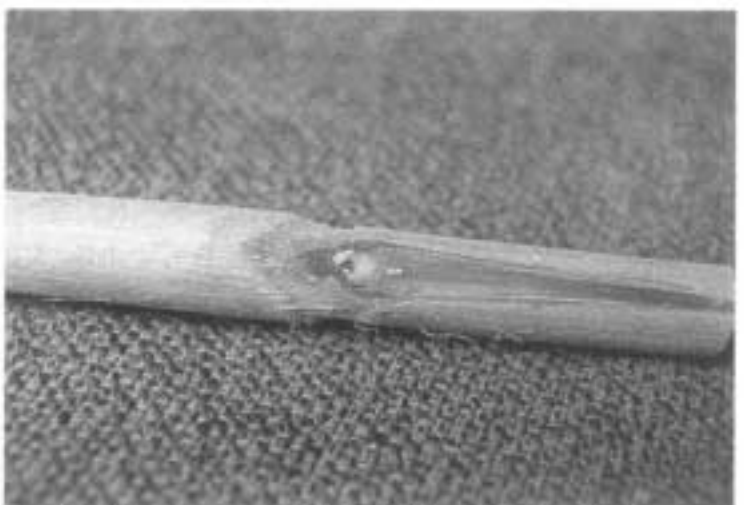
Fig. 25. Defective cane of Korthalsia sp. with nodal scar
