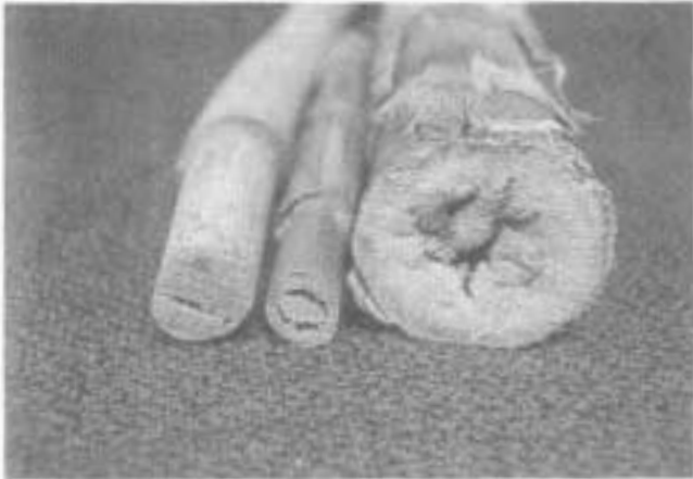
Fig. 26. Canes with shakes
