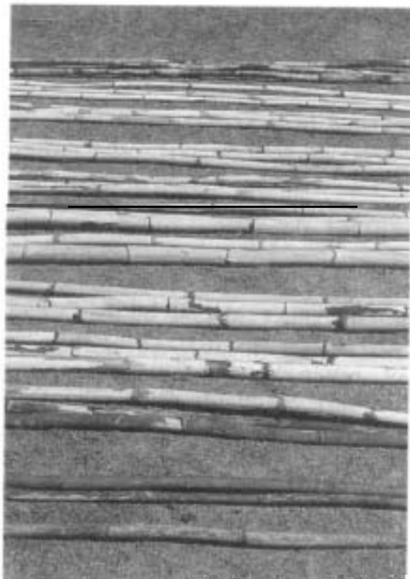
Fig. 11. Gradual change of skin colour from green to ivory-white in sun-drying of oil-cured rattan. Note the colour of untreated canes (top and bottom).
