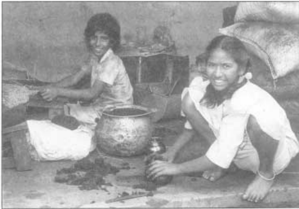
Fig. 4: Jigar and charcoal powder are mixed for preparing the thick paste for rolling agarbathi sticks
