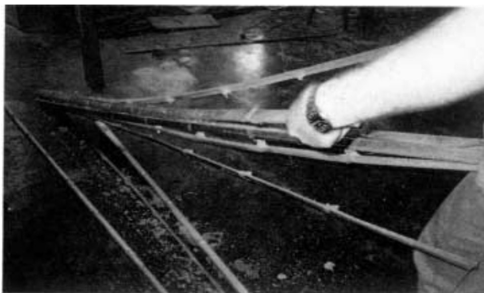
Fig. 12: Splitting a cut bamboo culm into narrow strips
