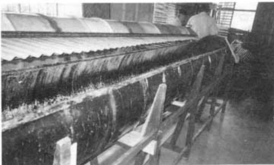
Fig. 14: Dip diffusion tank for preserving the bamboo tablilla
