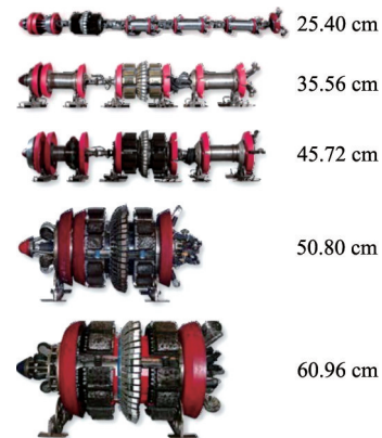
图4 威德福公司不同外径尺寸的MFL套管漏磁检测仪 Fig. 4 MFL casing leakage detecting instrument with different outer diameter
