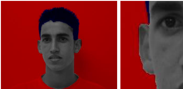
Figure 3. Example of automatic face region segmentation: red region is set of pixels classified as a background
