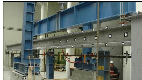
Figure 9. Long span HSC beams
