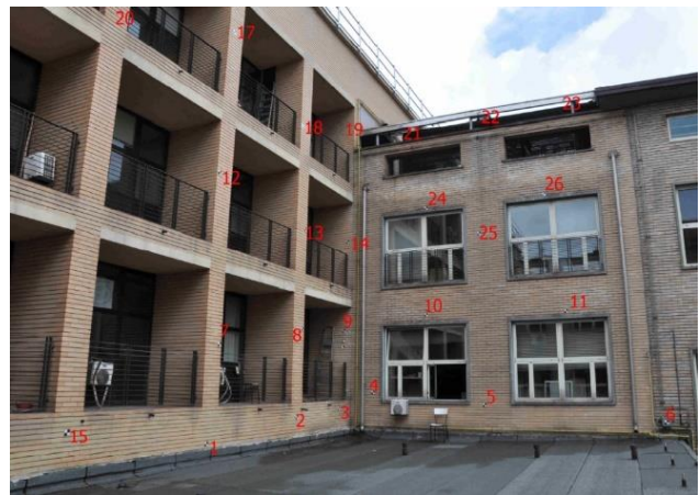
Figure 1. Calibration field for lens and sensors distortions
