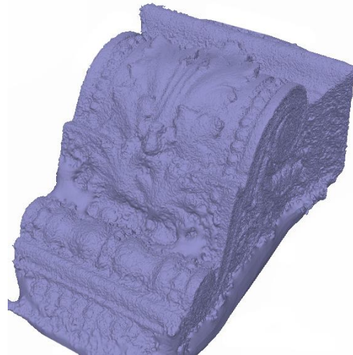
Figure 8 - Mesh of the iPhone point cloud
