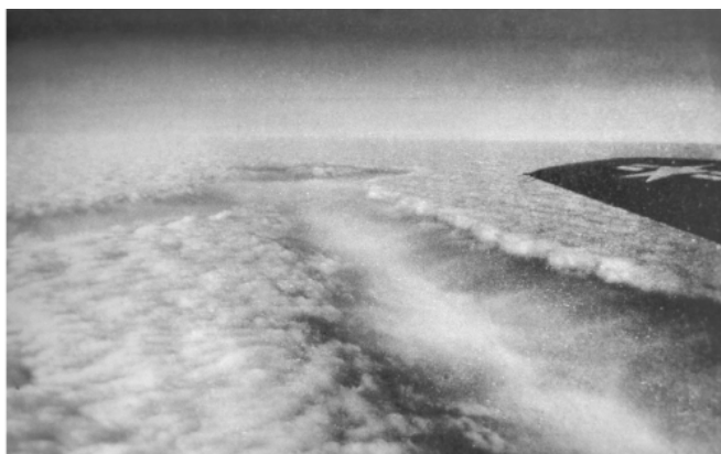
Figure 6.47. A \gamma -shaped path cut in a layer of supercooled cloud by seeding with Dry Ice. (Photo by courtesy of the General Electric Company, Schenectady, New York.)
