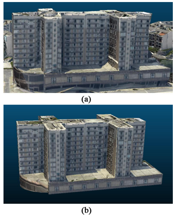
Figure 14. Comparison of our model with the manual model. The (a) is the 3D model generated in our method; (b) is the 3D manual model.
