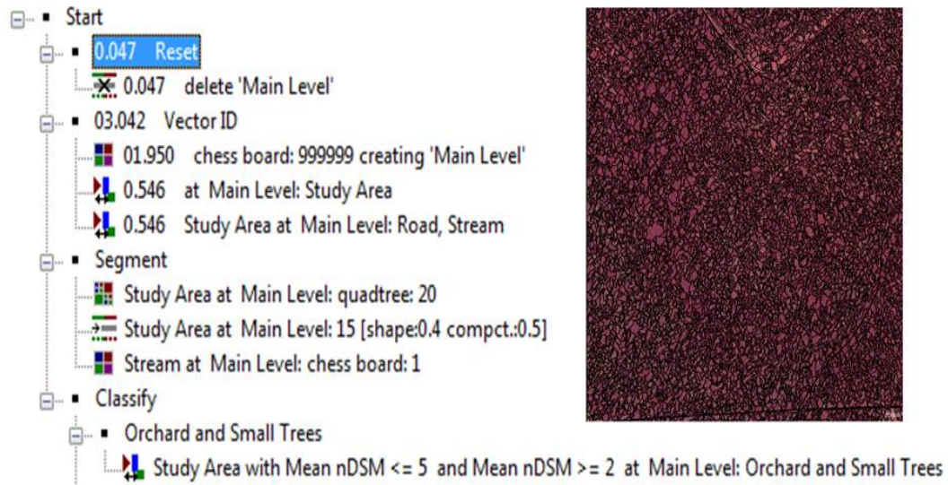
Fig 10a: Rule set to use tree height raster (nDSM) info for distinguishing orchards.
