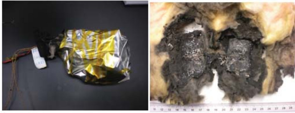
Fig. 4.10. The catastrophic results after thermal runaway happened
