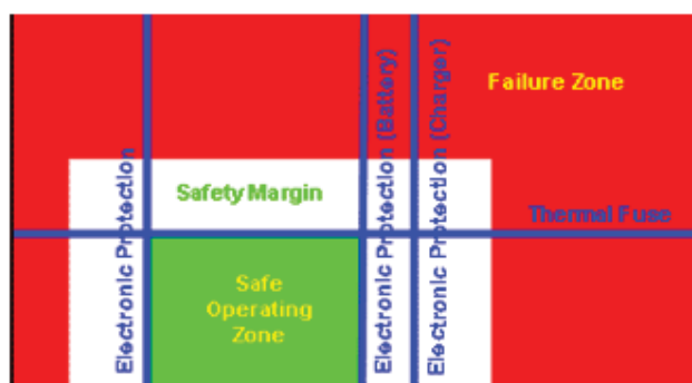
Fig. 1.10. Voltage based battery protection stratagem
