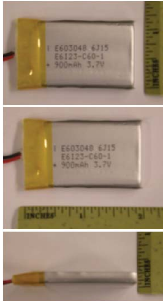
Fig. 4.1. The shape and size of the lithium-ion battery width, length and height
