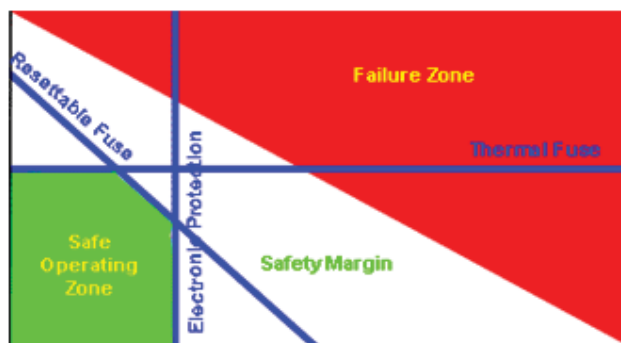
Fig. 1.9. Current based battery protection stratagem
