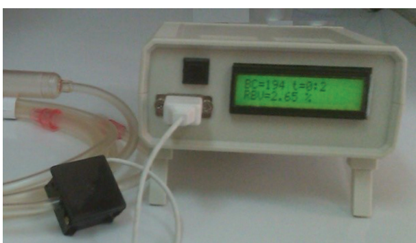
Figure 9. An Optical Device for RBV Measurement
