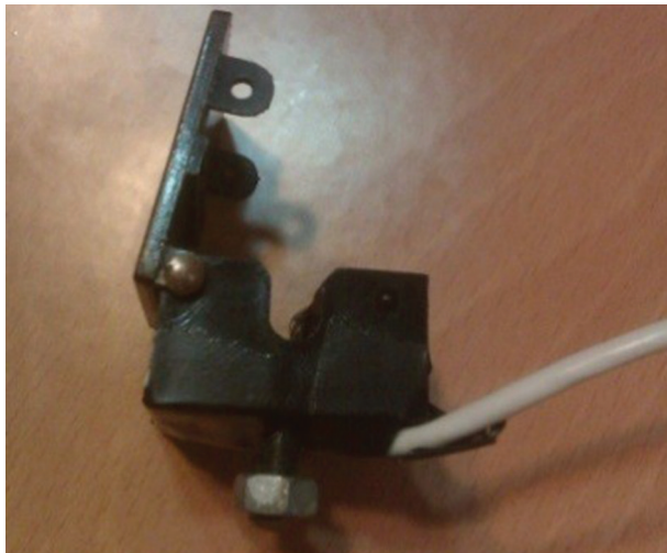
Figure 3. Prepared Sensor for Measuring the Blood Concentration
