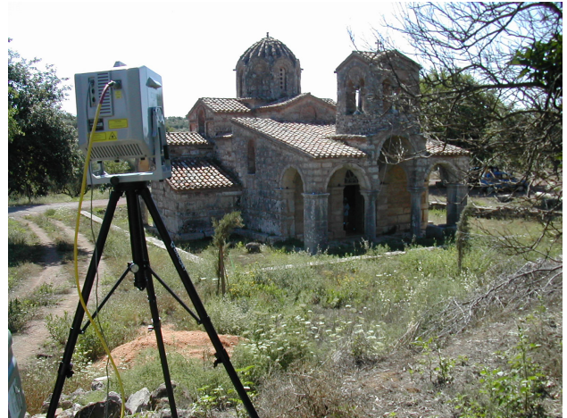
Figure 1. Agia Sanmarina and the Cyrax laser scanner. (By courtesy of ISPRS WG V/3)
