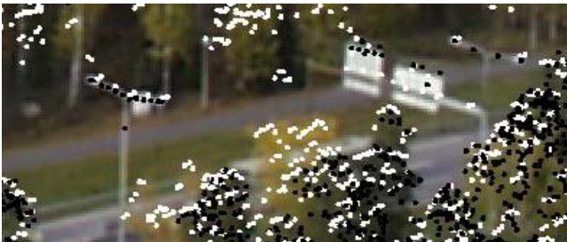
Figure 13. White spots (TopoSys-1) are scanned from 800 m with a pulse repetition rate of 83 kHz and black points (TopEye) are scanned from 200 m at a scanning rate of 7 kHz. (Rönholm et al., 2003)
