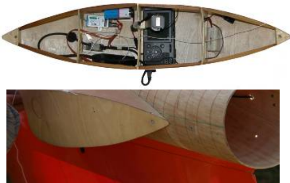
Figure 3. “Pod“ with Ricoh GR digital, and “pod” position under the UAV
