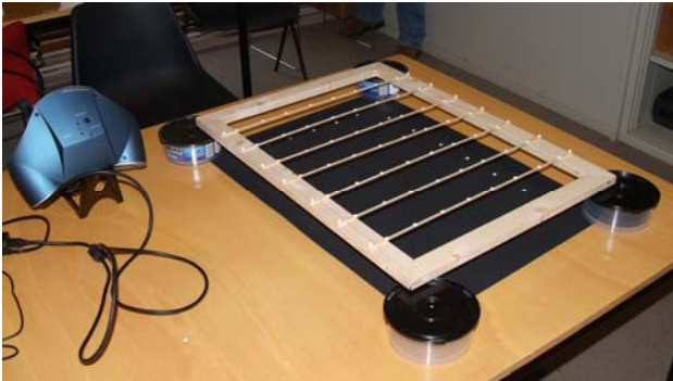
Figure 3: 3D grid of reflective targets
