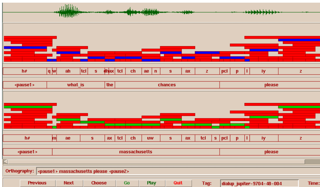
Figure 2: Example of the recognition result with and without reliability models in the JUPITER domain. The upper panel shows that, without reliability models, the utterance is incorrectly recognized as “what is the chances please”. The lower panel shows the result using the reliability models, and the utterance is correctly recognized as “Massachusetts please”.
