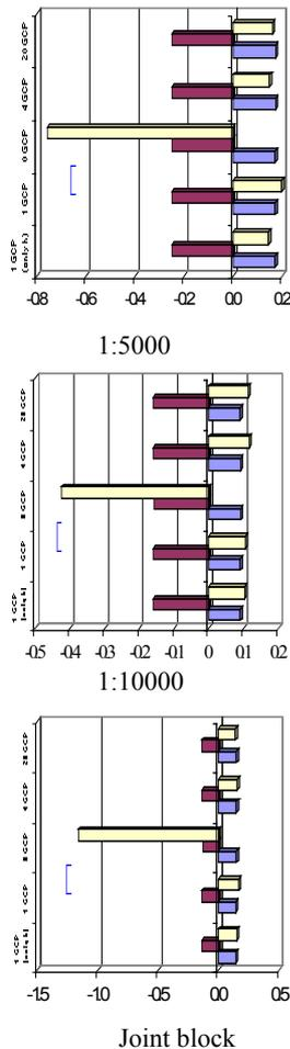
Table 2 shows the graphs for the estimates  $a$  vector components. It is apparent that while  $a_x$  and  $a_y$  are pretty stable, irrespective of the ground control,  $a_z$  does not and cannot be estimated without control points.
