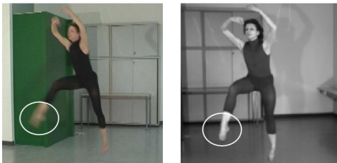
Figure 3. Comparison of motion blur at different frame rates: (a) SONY DCR-VX2000 camcorder at 25 frames/sec, and (b) Mikromak HCC1000 high-speed camera at 462 frames/sec.
