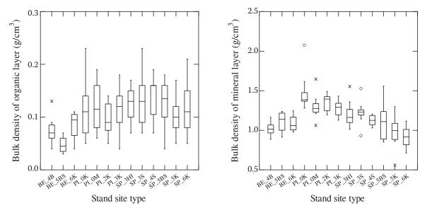
Fig. 4. The estimated bulk density for organic (left) and mineral (right) layer for the measured soil samples from 2004 stratified by stand site type
