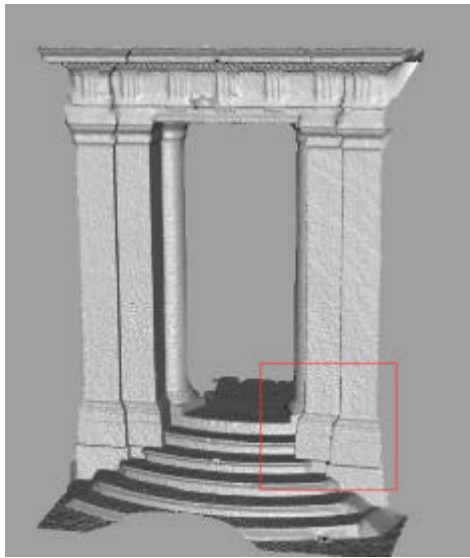
Fig. 8: Result obtained by TIN method ( software Paraform Points2Polys )
