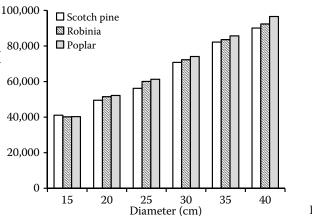
Fig. 2. Stump extraction force as a function of the stump diameter at the cutting plane
