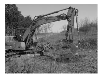
Fig. 1. Stump lifting by means of an extraction machine mounting one grab
