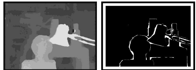
Figure 3: Disparities for Tsukuba (left) and differences to ground truth (right) – white: disparities more than 1 pixel too large; grey: disparities more than 1 pixel too small.
