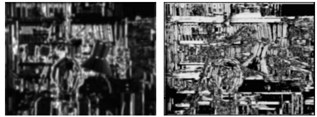
Figure 8: Horizontal gradient (left); Maximum auto-correlation along the horizontal line ranging from outside the matching window to the search width (right). Both images are slightly smoothed with a Gaussian.
