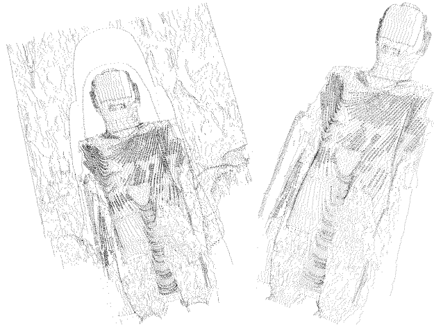
Figure 5: The point cloud of the manual measurement. The main edges and the structures of the folds, measured as breaklines, are well visible
