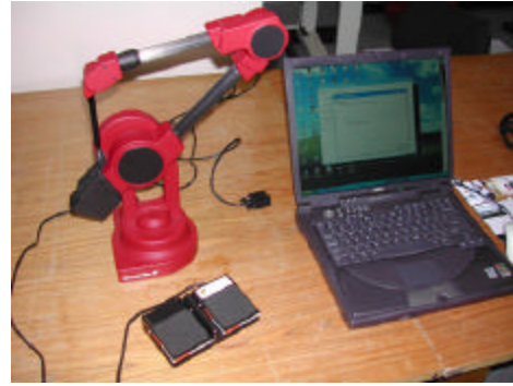
Fig. 2: MicroScribe Digitiser, its accessories and the laptop
