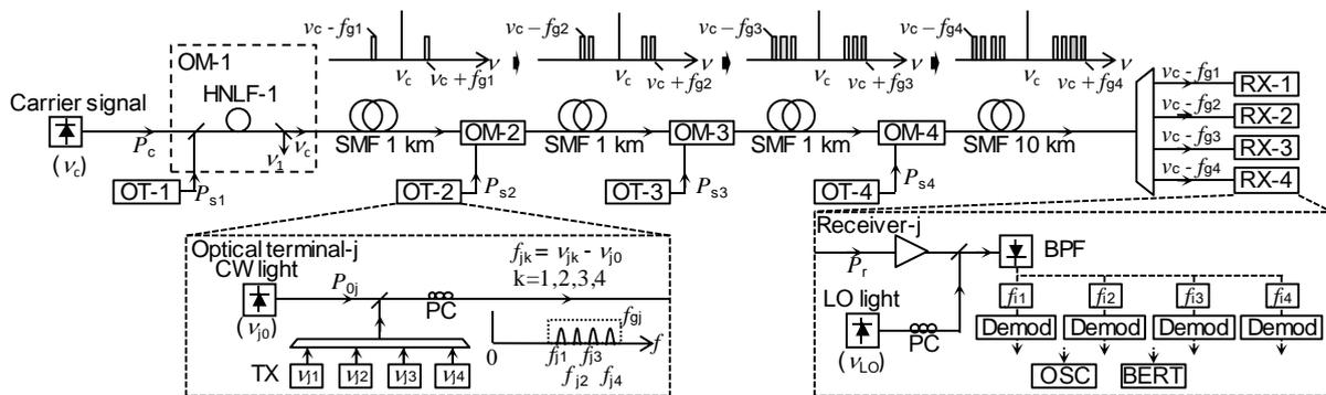
Fig. 2. Experimental setup of 4-stage multiplexing
