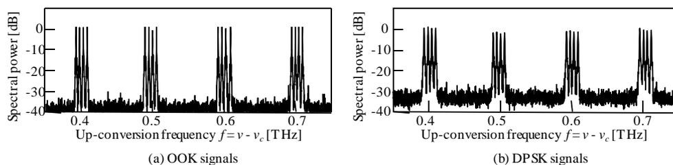
Fig. 5. Optical spectrum of 16-ch multiplexed signals.
