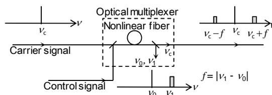
Fig. 1. Optical multiplexer by fiber XPM
