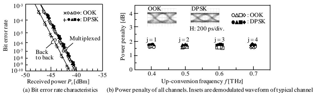
Fig. 6. Bit error rate characteristics (a), and the measured power penalty (b), after 10-km transmission.
