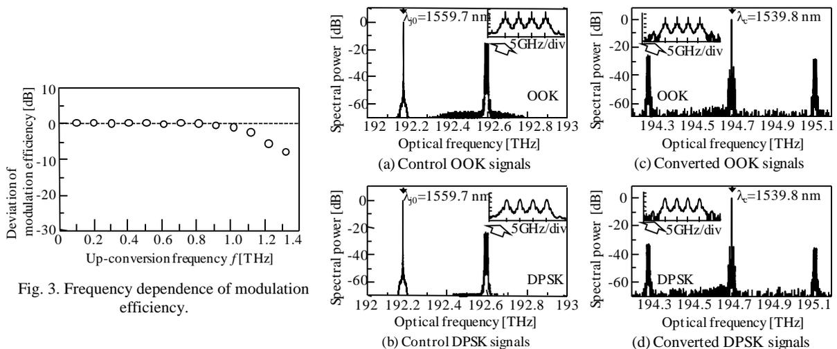
Fig. 3. Frequency dependence of modulation efficiency.
