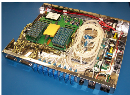
Fig. 6. 19 inch rack mounted PLZT 4x4 switch.
