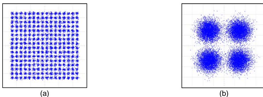
Fig. 6: Received constellations: 256QAM, subcarrier's number 1-16 (a); 4QAM (b), subcarrier's number 197-256
