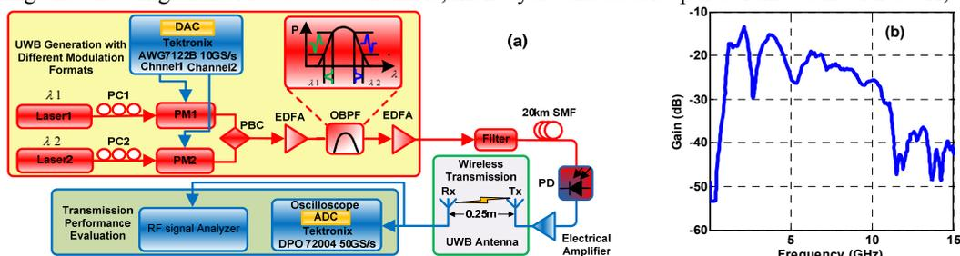
Fig. 1. (a) Experimental setup of the UWB over fiber system reconfigurable for different modulation formats (b) Frequency response of the lab-made UWB antennas pair with a distance of 0.25m
