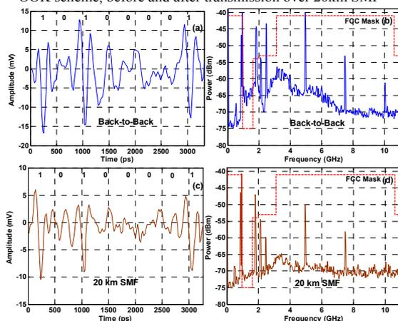
Fig. 4. Temporal waveforms and electrical spectra of doublet OOK scheme, before and after transmission over 20km SMF
