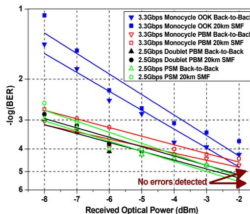
Fig. 7. BER measurements of UWB over fiber system with OOK, PBM, and PSM before and after 20km SMF transmission
