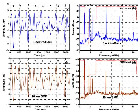
Fig. 6. Temporal waveforms and electrical spectra of PSM scheme, before and after transmission over 20km SMF
