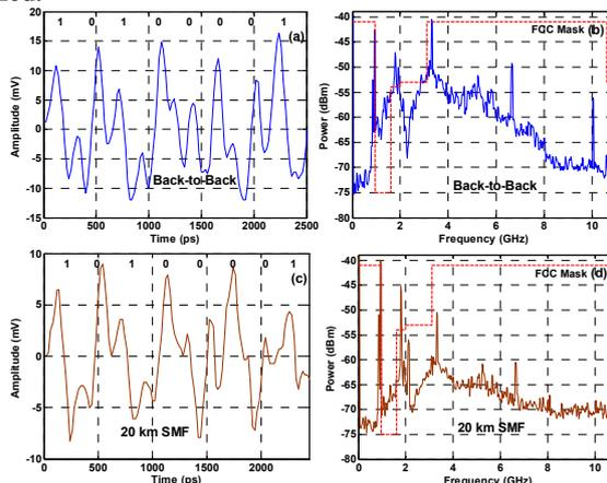
Fig. 3. Temporal waveforms and electrical spectra of monocycle PBM scheme, before and after transmission over 20km SMF
