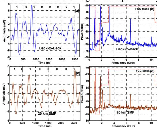
Fig. 2. Temporal waveforms and electrical spectra of monocycle OOK scheme, before and after transmission over 20km SMF
