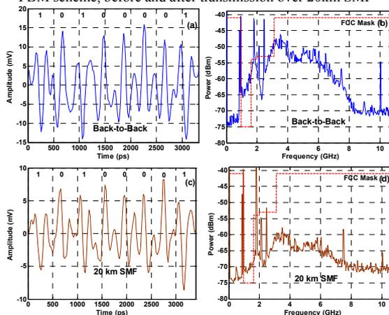
Fig. 5. Temporal waveforms and electrical spectra of doublet PBM scheme, before and after transmission over 20km SMF
