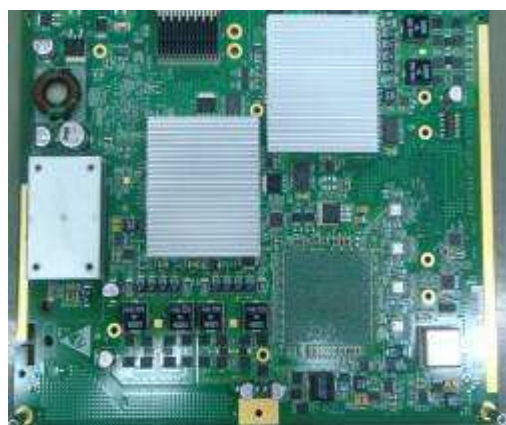
Fig. 3. One FPGA board of the emulator system
