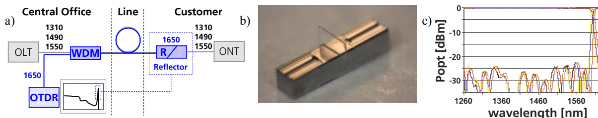
Fig. 2 (a) OTDR monitoring of passive optical networks; (b) OTDR PolyBoard; (c) spectrum of bare T2FE
