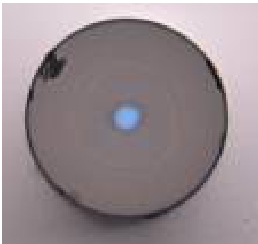
Fig. 2. Photograph of the cleaved end with a 12-μm-diameter core.
